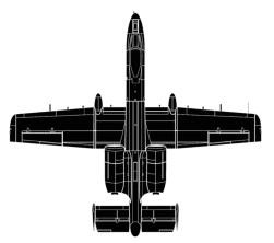
The A-10 Thunderbolt II dates to 1967, when USAF began an A-X program to develop a dedicated close air support aircraft. The service wanted its new fighter to be uncomplicated, able to absorb massive battle damage, easy to maintain, operable from unimproved strips with heavy ordnance loads, and cheap. Speed and sleekness were not must-haves. The result-Fairchild Republic's plain but now-famous Warthog-proved to be all the Air Force wanted, and more.
